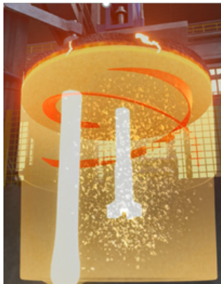
Very fine Ar bubbles helically dispersed
