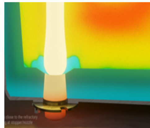
Cold spots of metal after the tapping
